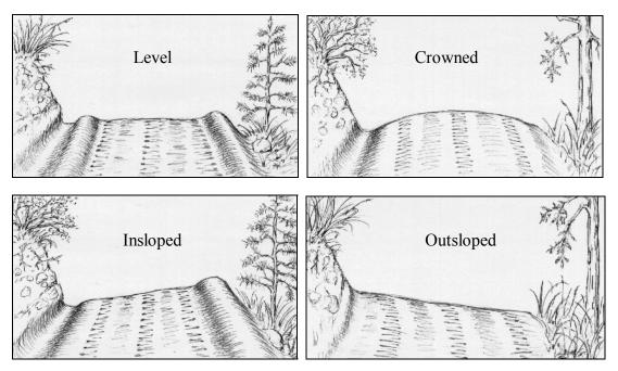
Figure 5-4. Road Drainage Designs
