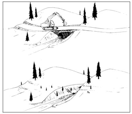
Figure 5-1. Removing a Road Crossing
