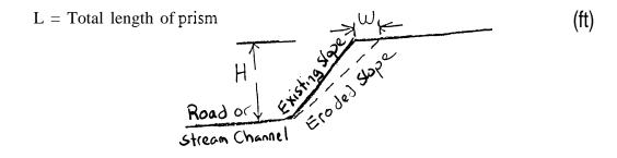
$$\underline{Gu} \qquad \underline{(D)epth*(Width*(L)ength)} = Erosion Volume (cu. yds.)$$
