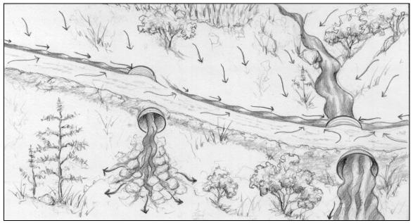
Figure 5-9. Road Drainage Issues Affecting Stream Channel Stability
